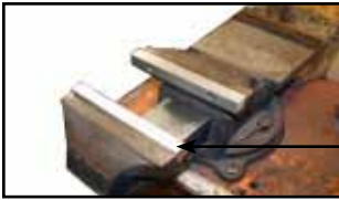
A Soft - Jaw vice (Aluminum or Copper Jaws)
