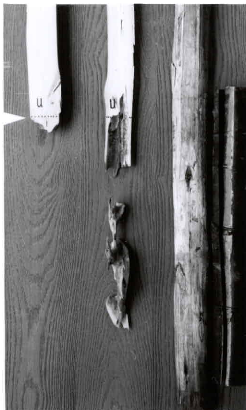
Fig. 3. Untreated poles after 6 months' in soil-contact showing that unsleeved poles (left and centre) were mineralised below the ground line (arrowed), whereas sleeved poles (right) were not.
