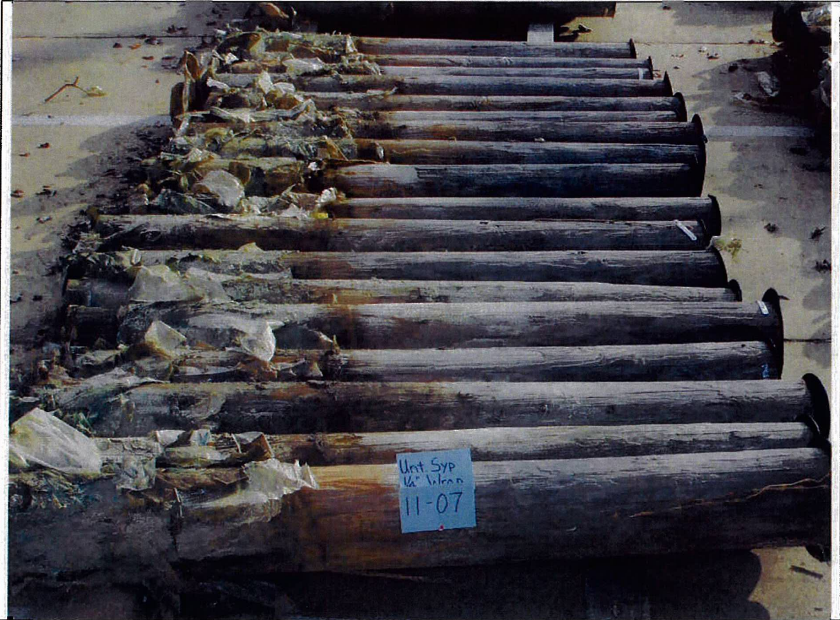
Figure 4 - Group photo of untreated pine pole stubs which received a supplementary wrap/bandage 1/4" thick.
