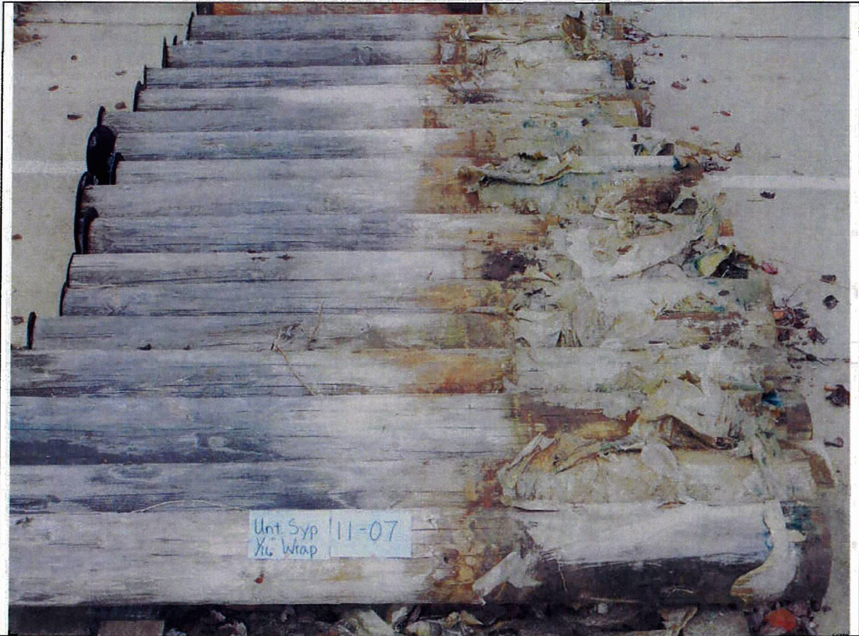
Figure 2 - Group photo of untreated pine pole stubs which received a supplementary wrap/bandage 1/16" thick.
