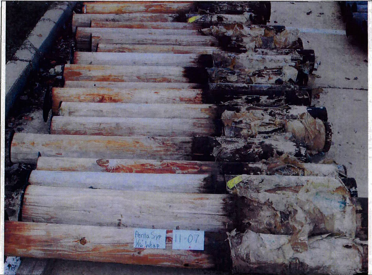
Figure 6 - Group photo of penta treated pine pole stubs which received a supplementary wrap/bandage 1/16" thick.
