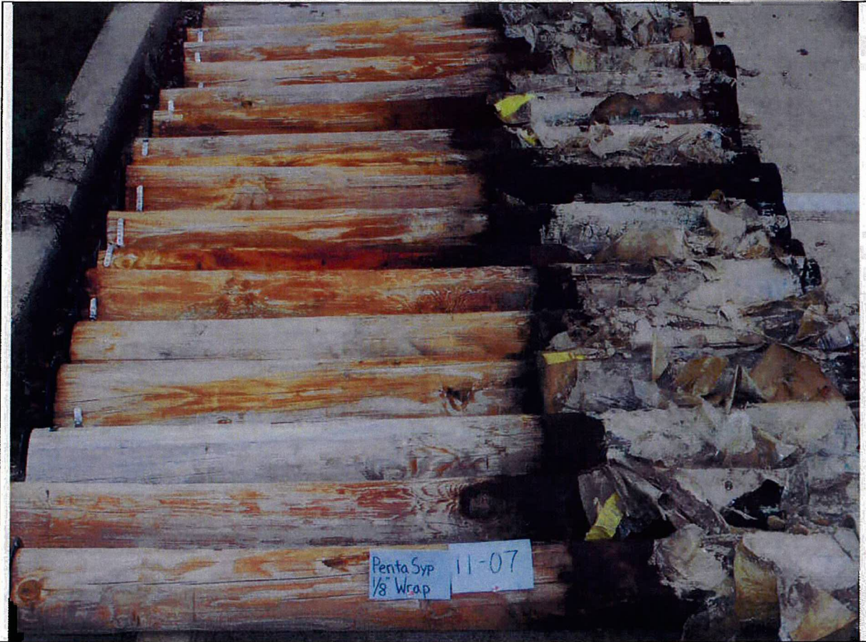
Figure 7 - Group photo of penta treated pine pole stubs which received a supplementary wrap/bandage 1/8" thick.
