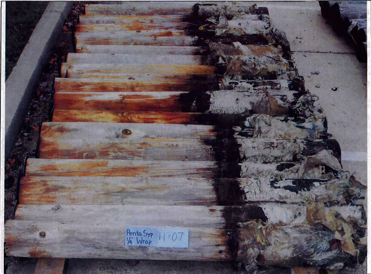
Figure 8 - Group photo of penta treated pine pole stubs which received a supplementary wrap/bandage 1/4" thick.
