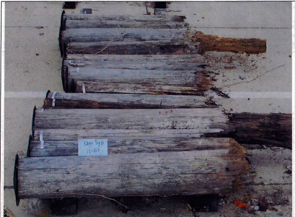
Figure 1 – Group photo of untreated pine pole stubs which did not receive a supplementary wrap/bandage.
