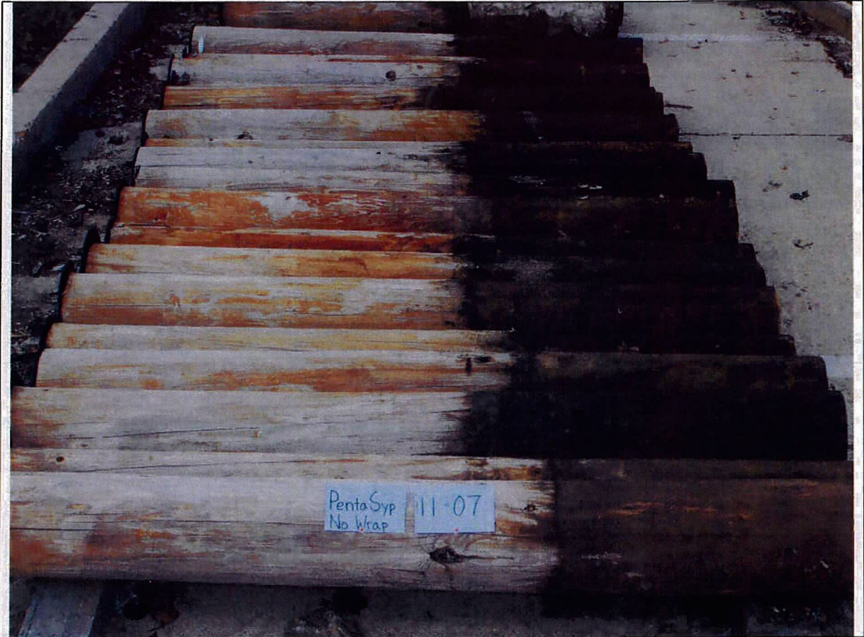
Figure 5 – Group photo of penta treated pine pole stubs which did not receive a supplementary wrap/bandage.
