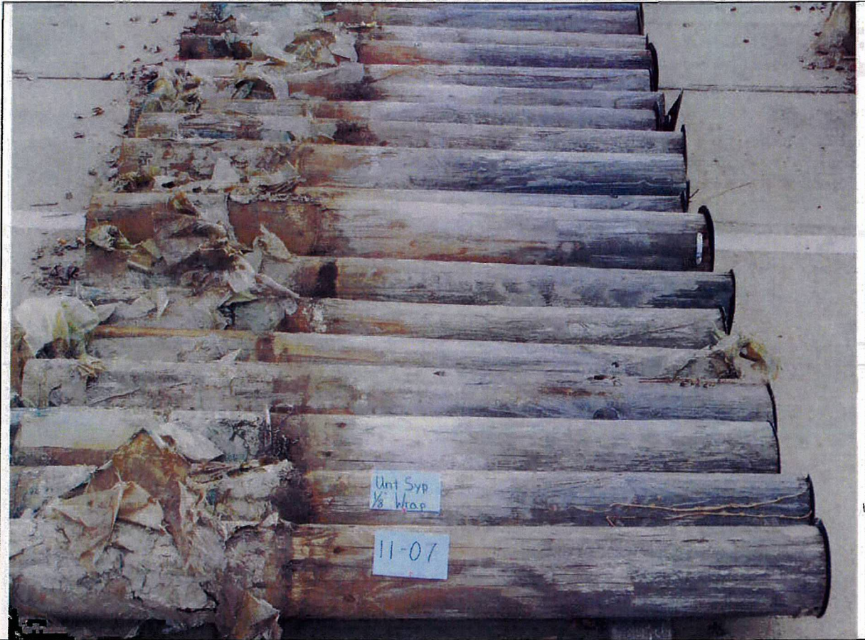
Figure 3 - Group photo of untreated pine pole stubs which received a supplementary wrap/bandage 1/8" thick.
