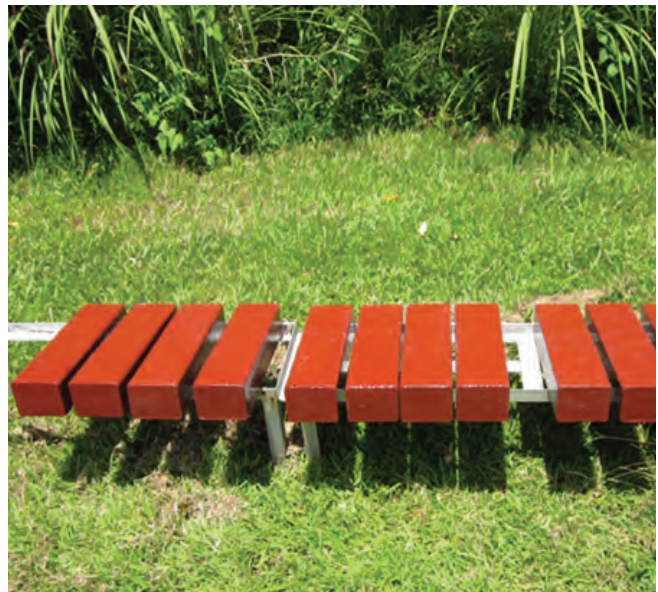
Figure 28. Polyurea-coated arms designed to reduce the risk of checks developing on the upper surface.
