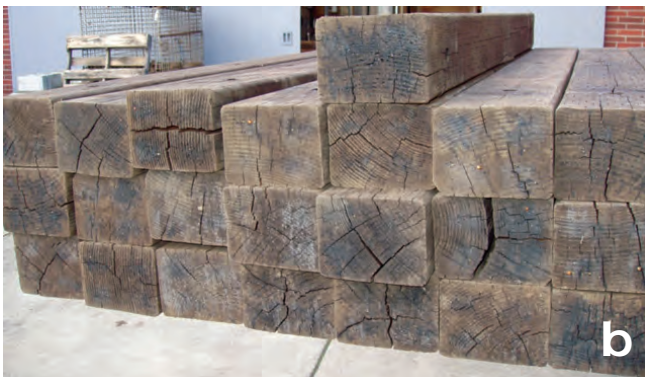
Figure 27. Crossarms (a) with and (b) without end-plates that limit end-checking. Note the large checks on non-plated ends.
