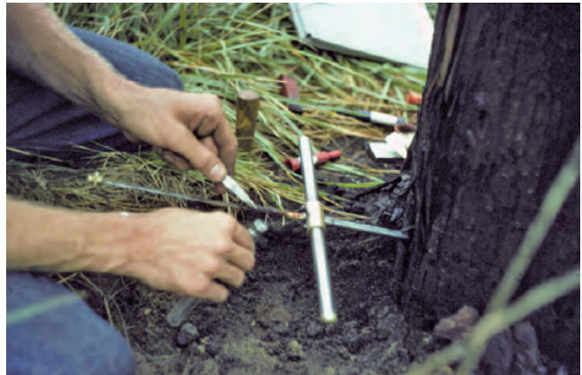
Figure 35. Cores extracted with an increment borer permit detection of rot, as well as measurement of shell thickness and depth of preservative penetration. Cores can be retained and cultured for fungi.
