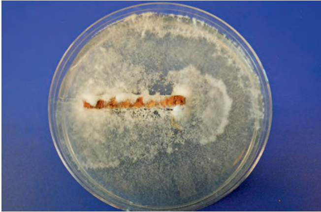
Figure 17. A decay fungus growing over malt agar from a sound-appearing increment core is a positive sign of decay, even though the pole may contain no visible rot.
