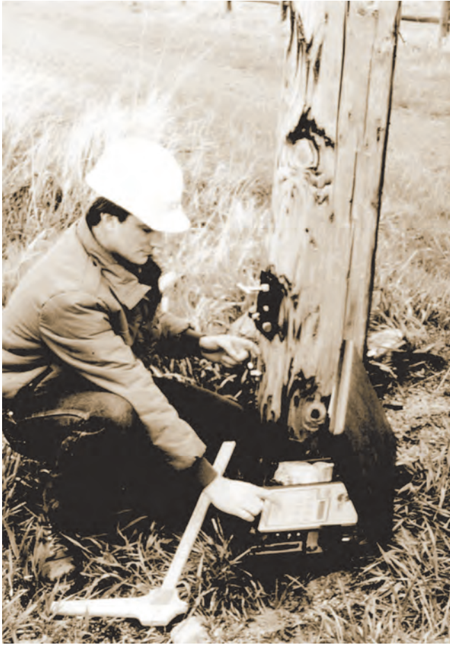
Figure 41. Pole test with an acoustic inspection device.
