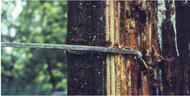
Figure 36. A shell-thickness indicator detects rot in poles by “feeling” growth rings in sound, but not rotten, wood when inserted or removed from snug-fitting holes.
