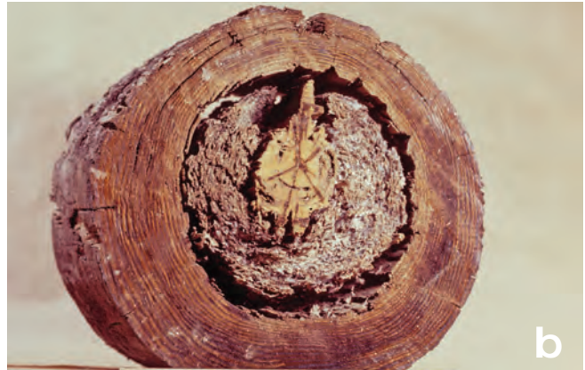
Figure 19. A termite colony includes many workers that burrow in wood for food and shelter, soldiers that protect the colony from other insects, and one egg-laying queen. (a) These reproductives later will fly from the nest to initiate new colonies (photo credit: Scott Bauer, USDA Agricultural Research Service, Bugwood.org). (b) Usually poles show no sign of termites until the reproductives emerge, discard their wings, and mate to start new colonies (photo credit: Gerald J. Lenhard, Louisiana State University, Bugwood.org).
