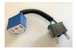
Depending on the low beam/high beam configuration that you want, the adaptors can be modified by using a small paper clip or other small pointed object to move pins to a different location on the socket.
