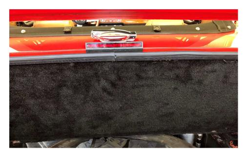
7. The Auxiliary light can be connected as an additional running light or as a brake light.
