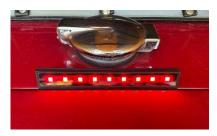
The Auxiliary light can be connected as an additional running light or as a brake light and is designed to fit in the rain gutter of the Triumph TR6 trunk. The light housing is ABS plastic with red lens, a 9 LED strip, double back sticky pads for mounting and approximately 6 ft of two conductor wire terminated for installation.
